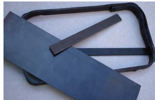
Figure 2-9: FRP plate and strips
